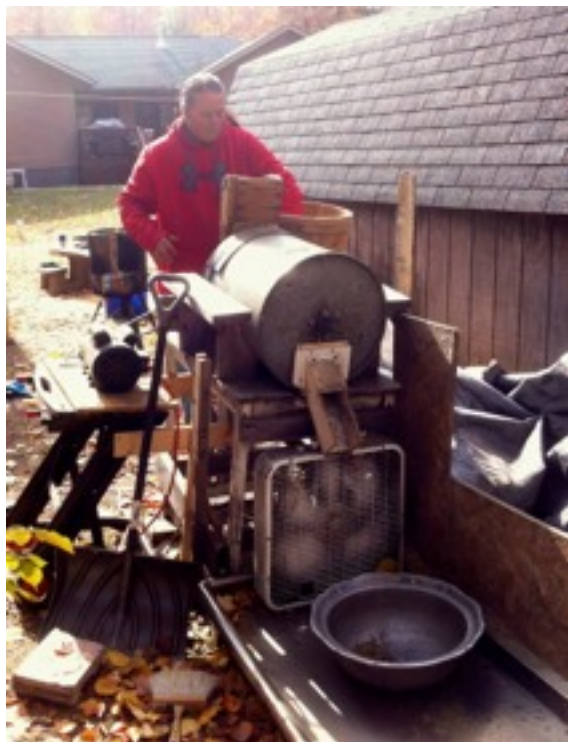
Figure 1: Wayne Valliere using Leon Valliere's homemade wild rice hulling machine.
