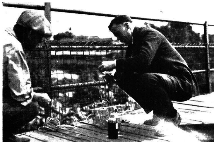
An important factor in the control of stream pollution is the oxygen content. These men are finding the oxygen content at Rhinelander, Wisconsin.
