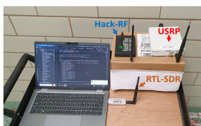
Fig. 6.6: 3 Software Defined Radios as Base Stations
