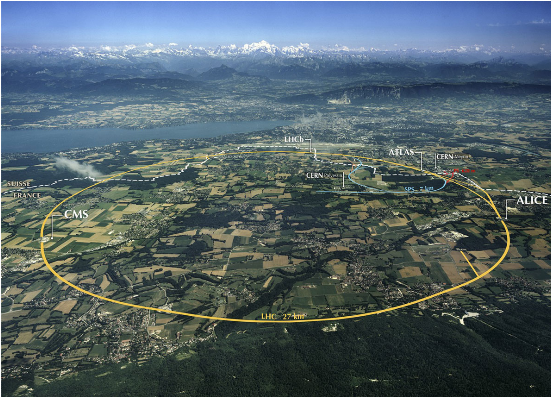
Figure 2.1: The Large Hadron Collider at the French/Swiss board. The yellow ring indicate the LHC ring, which is 50 m to 100 m underground. Locations of the four main experiments are shown on the plot. The detector for each experiment are inside the LHC tunnel. Location for the SPS and PS are also shown [99].
