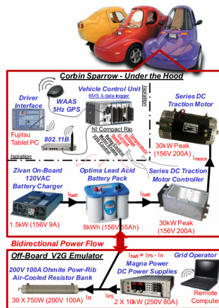
Figure A 2 WEMPEC Corbin Sparrow system diagram [140]
