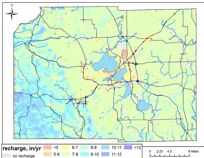
*Fig. 10. Calibrated steady-state recharge distribution in inches per year. Highest estimated recharge rates occur within the Driftless Area while the lowest recharge rates are in urban settings with concentrated areas of impervious cover. As an example, the Dane County regional airport, located north of Madison and east of Lake Mendota, is a distinctive area with reduced recharge visible at the county scale (from Parsen et al. 2015).*
