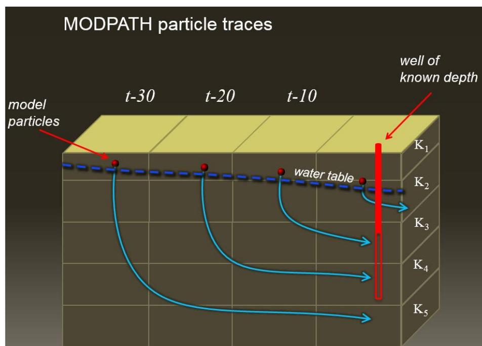
*Fig. 11. Generalized illustration showing MODPATH particle tracking from the water table to a well of known depth. The open interval of the well is shown as lower hollow portion of the well. The hydraulic properties of each model layer are denoted by the range of K-values, while the back-calculated travel times from the open interval of the well back to the water table are denoted with the time range t-10 to t-30 years.*
