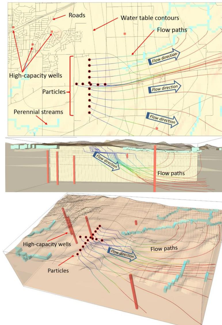
*Fig. 4. Example showing particle tracking using MODPATH with MODFLOW. Particle pathways illustrate the three-dimensional movement of groundwater flow and allow for detailed spatial analysis of simulated flow through the groundwater system (from Bradbury 2015b). The changing colors of flow paths indicate the relative travel time or age of groundwater from blue (young) to red (old).*
