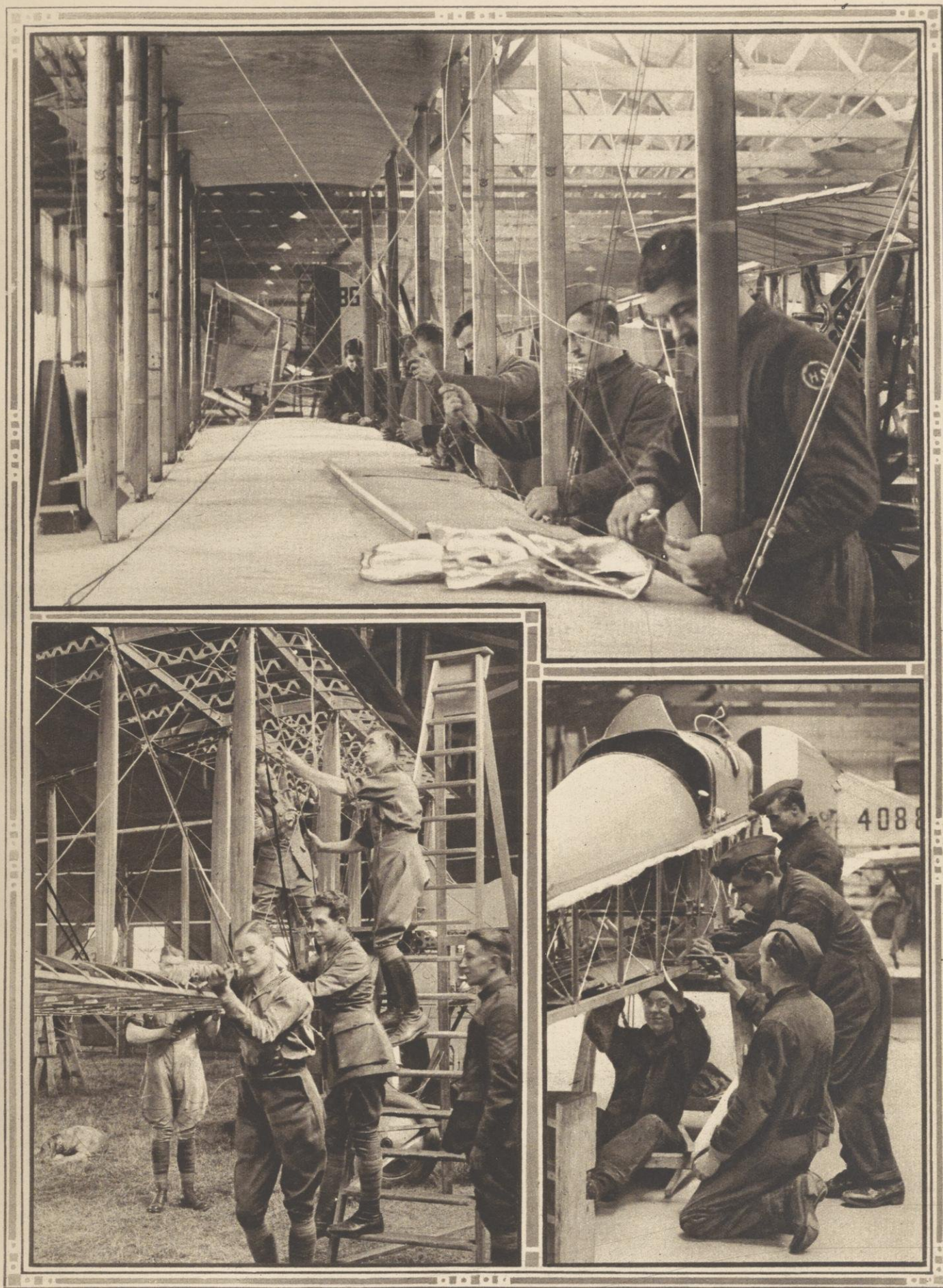
INSTRUCTION IN RIGGING AN AEROPLANE. PHOTOGRAPHS SHOWING THE WIRING OF A MACHINE.
