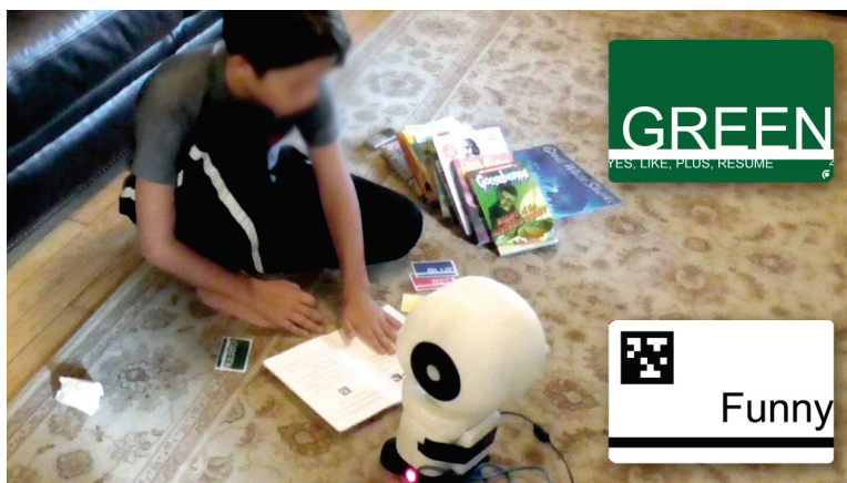
Figure 4. Image of a child working with Minnie during the introductory process. The child is holding a topic interest card and has placed the “Talking with Minnie” book on the floor in front of Minnie. The books available for the child to read appear on the right of the image. An example of a green RFID card (top) and a topic interest card with an April tag (bottom) are superimposed on the right of the figure.
