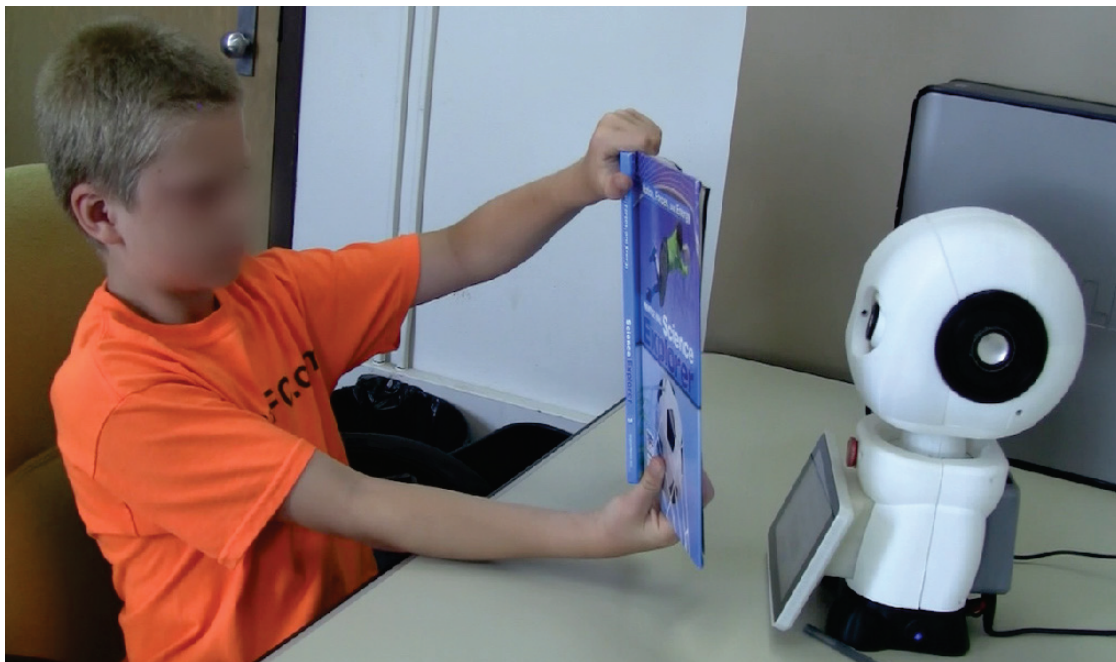
Figure 11. Child scanning an AprilTag with the redesigned Minnie robot, by pointing the textbook towards the robot’s camera (red circle on robot torso).
