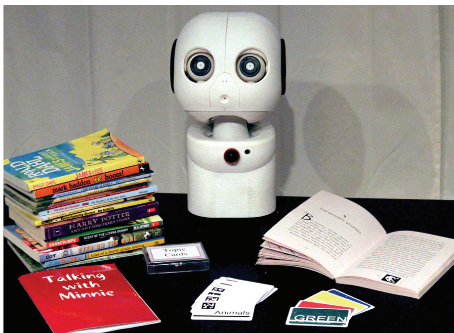
Figure 3. Image of the learning companion robot, Minnie, used in the study as well as the introductory “Talking with Minnie” book, RFID topic and interaction cards, and books augmented with AR tags. The robot’s camera is the red circle on the upper torso. The RFID reader is below the camera and indicated by a red light when the robot is on.
