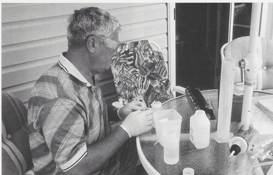
Bob Gayhart tests oxygen and phosphorus levels which indicate how well lakes can support fish and aquatic bugs as well as measuring how fast the lake is aging.
