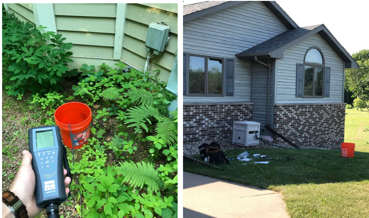
Figure 4. Measuring field parameters using YSI Professional Plus multiparameter instrument at location L3 (left), 1-hour pump test at location L9 (right).
