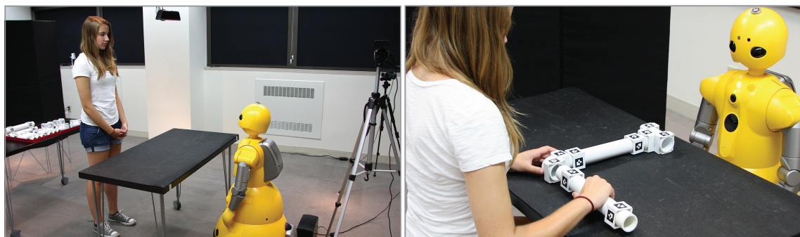
Figure 5.3: On the right, the setup used in my experimental evaluation. After the robot gave an instruction, the participant retrieved the pieces necessary from behind them and assemble the pieces on the workspace in front of the robot. A camera above the workspace captured the configuration of the pieces. On the left, an example of the robot autonomously guiding a participant in assembling pipes.
