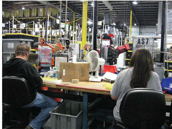
Figure 3.4: Two operators working near the robot. The vantage point of the operators makes it difficult to monitor the robot's status. Additionally, the tasks the operators are completing requires their visual attention.
