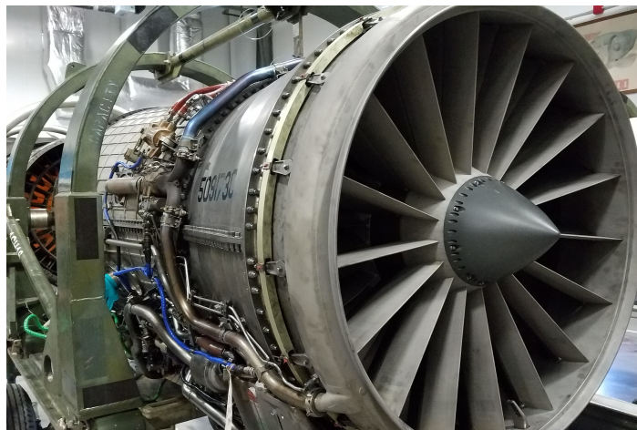
Figure 1: GE F110 engine for the F-16 (image courtesy of Prof. Matt Allen)
