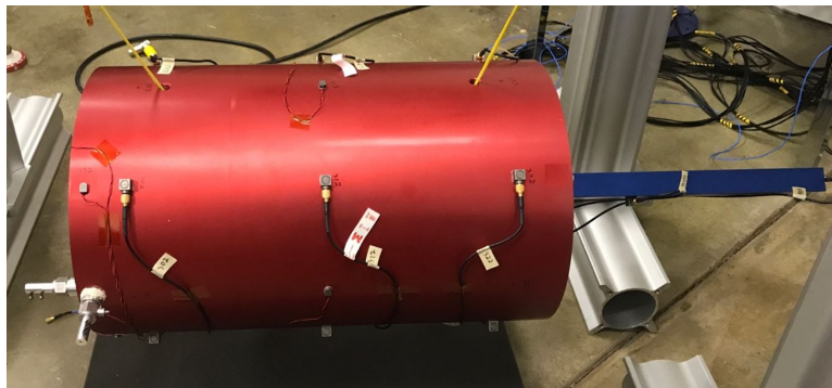
Figure 2: A side view of the Cylinder – Plate – Beam (CPB)
