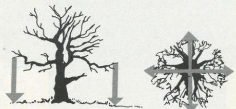
Crown spread is determined by setting out stakes at points of greatest and smallest spread, measuring the distance between them, and taking an average.
