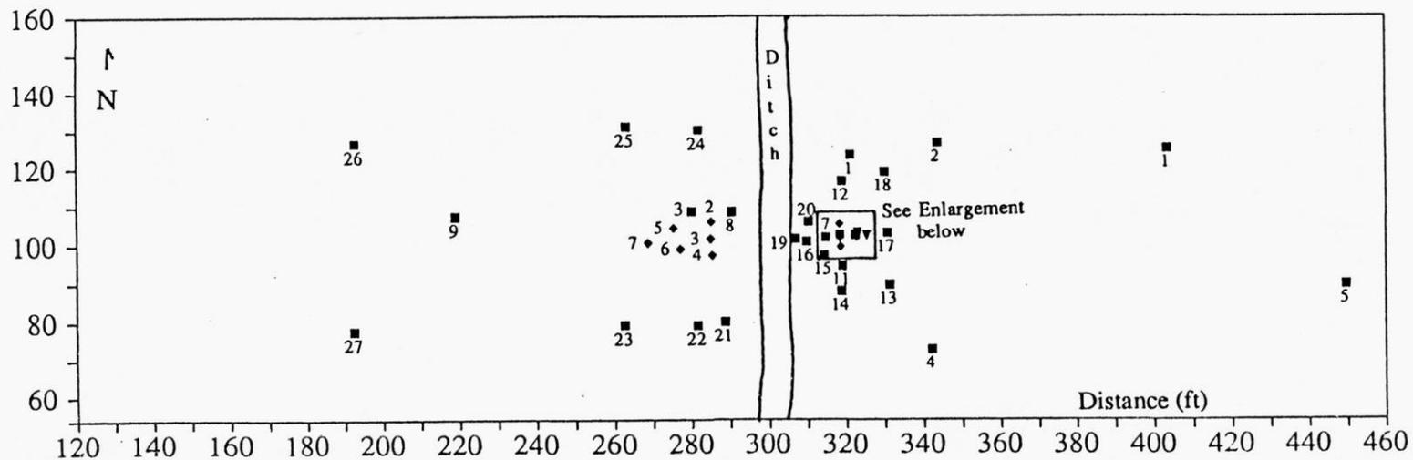
Figure 3.1 Location of all wells installed at the field site in the fall of 1988. The squares represent water table wells (Wt), the triangles represent injection wells (IW) and the diamonds represent multilevel sampling wells (MI). The expanded view of the area near the injection wells shows the flow path of the tracer plume in the first tracer test.
