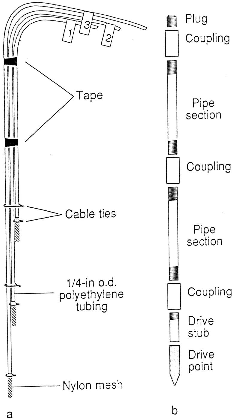
Fig. 1.a. Miniature multilevel sampling well. b. Exploded view of drive point and pipe assembly for miniature multilevel well installation.
