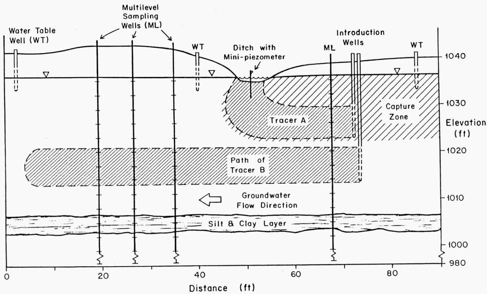
Figure 1.3 Schematic of the tracer test design.
