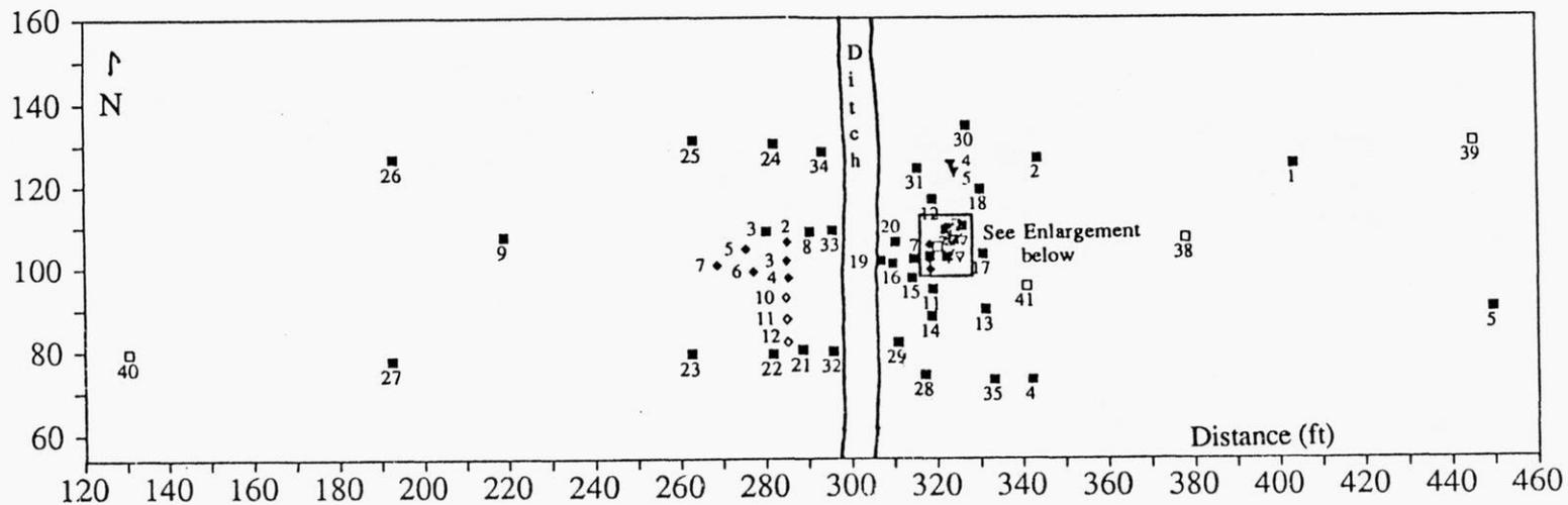
Figure 3.3 Location of all wells installed at the field site in July, 1989. The squares represent water table wells (Wt), the triangles represent injection wells (IW) and the diamonds represent multilevel sampling wells (MI). The open squares, triangles and diamonds represent well that have been added since the previous May, 1989. The enlarged area shows the many injection wells which were installed for tracer test 4.
