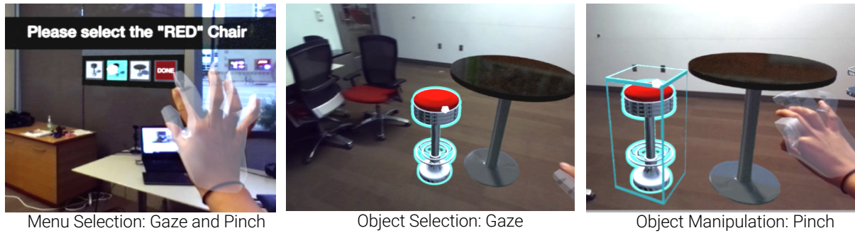
Figure 5.3. Gaze and Pinch Interaction: target the menu with gaze and accomplish the selection task by releasing an index finger (left). Select the virtual object with a gaze (middle) Hold a pinch gesture to move the object around (right)
