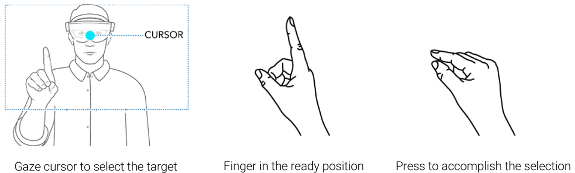
Figure 5.4 Illustration of two core inputs of Microsoft HoloLens: Gaze (left) and air-tab hand gesture 1
