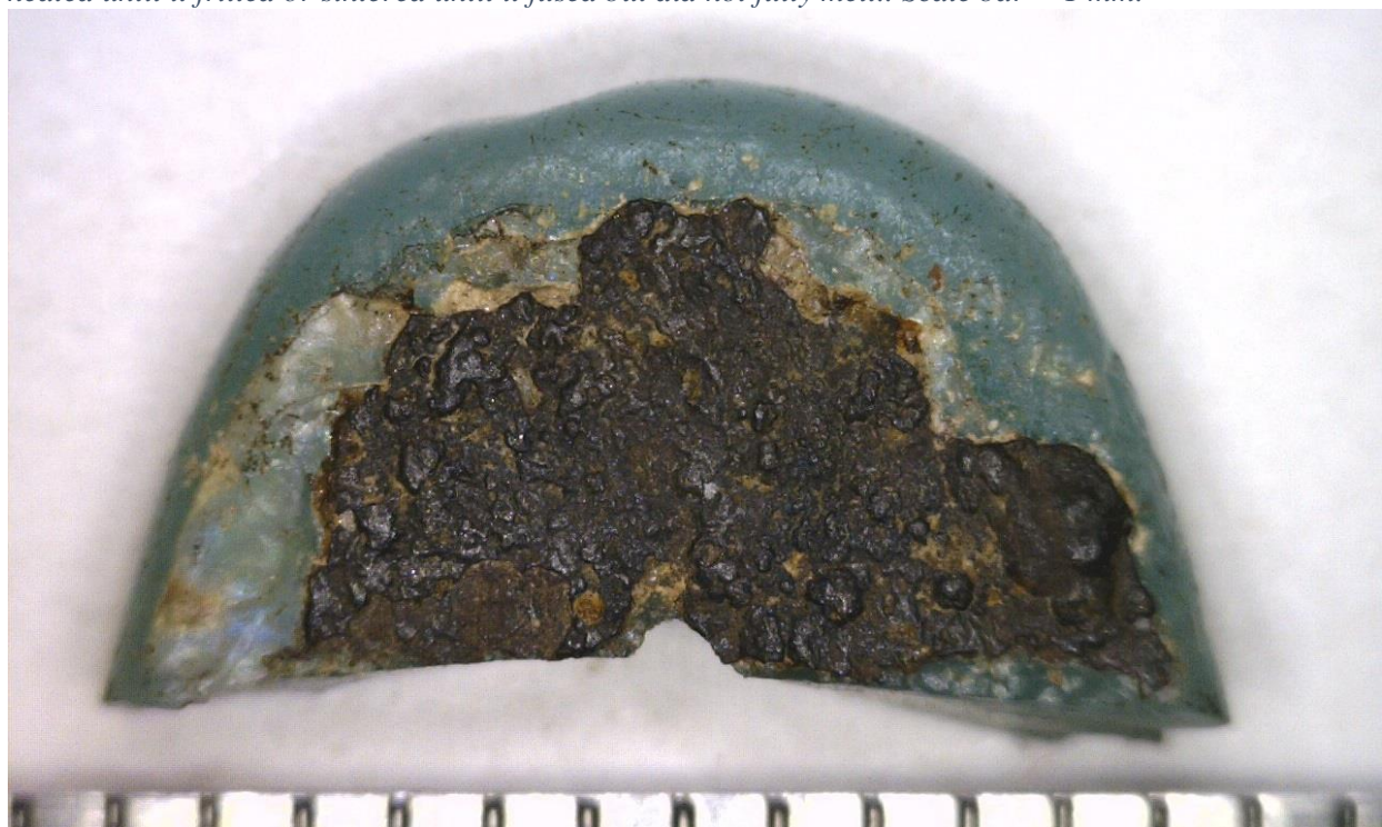
Figure 5.25: Interface between blue and white glass stripes of a glass pendant, showing grains of glass, heated until it fritted or sintered until it fused but did not fully melt.. Scale bar = 1 mm.
