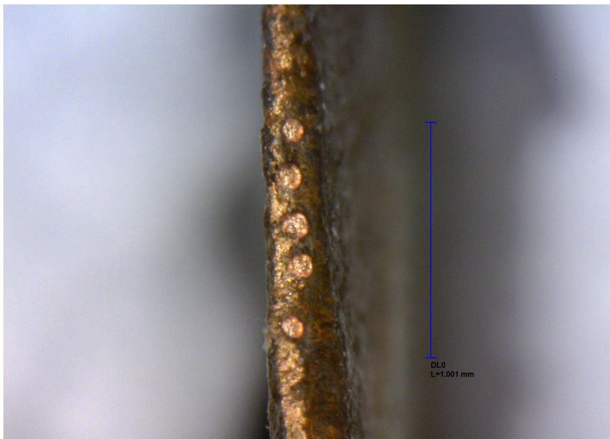
Figure 4.7 The cut edge of a copper object, showing five laser-ablation removal areas
