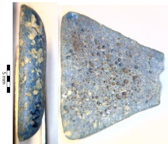
Figure 5.28: Pendant sampled in CM_73 and CM 74 illustrating the flat “back” of the pendant with bubbles or air pockets from heating, and the rounded profile of the object, which could result from partial melting or intentional shaping of the cooling glass paste.
