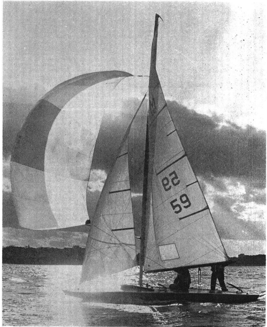
This U.W. Hooper Club M-20 is shown flying a "chute" or spinnaker. The jib and mainsail are well trimmed to get the most speed for the given wind direction.
