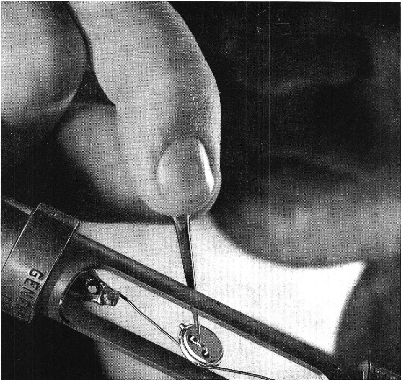
This RCA scientist points a tweezer at an experimental FM radio transmitting gallium arsenide device so small it is almost invisible.
