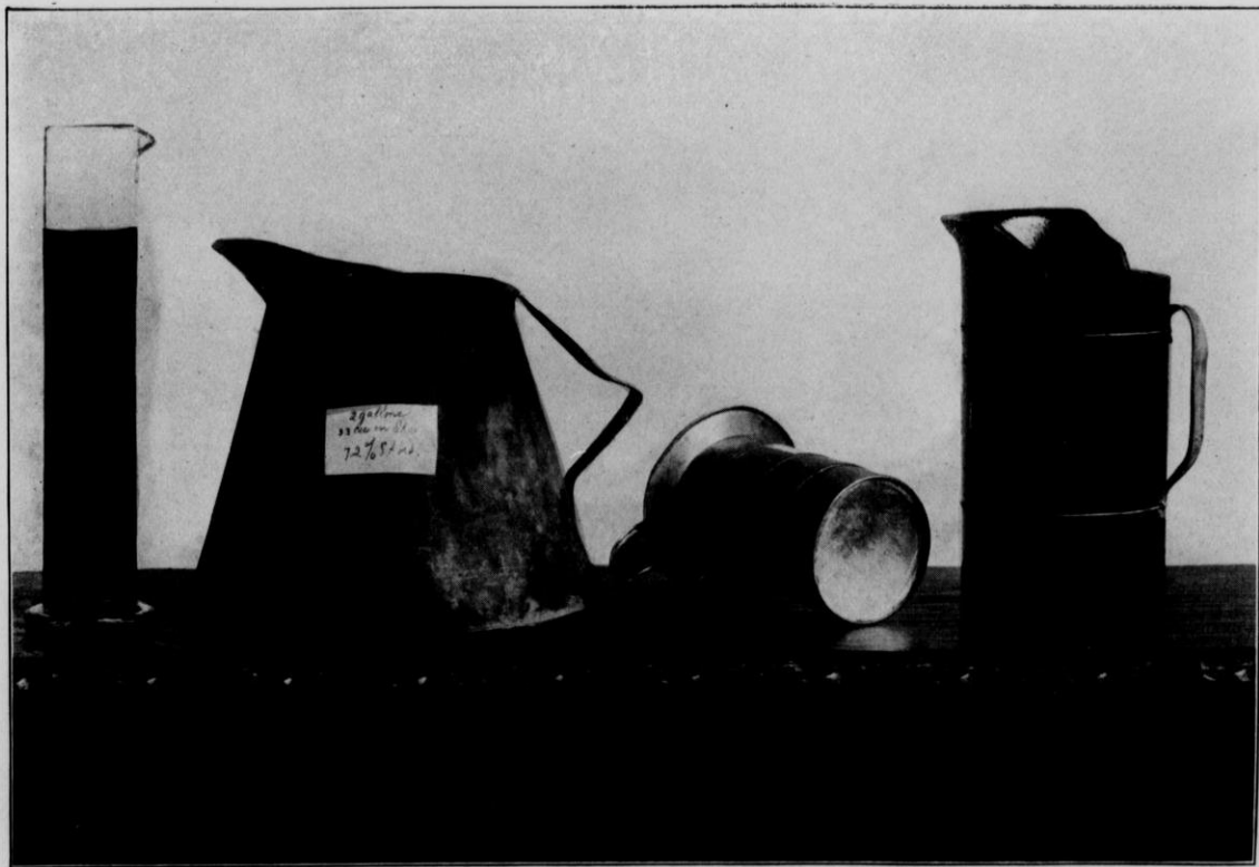
FIG. 20.—KEROSENE MEASURE, SHORTAGE SHOWN BY GRADUATE. MILK MEASURE WITH BOTTOM HAMMERED UPWARD. VINEGAR MEASURE MADE SHORT BY SAWING OFF TOP.
