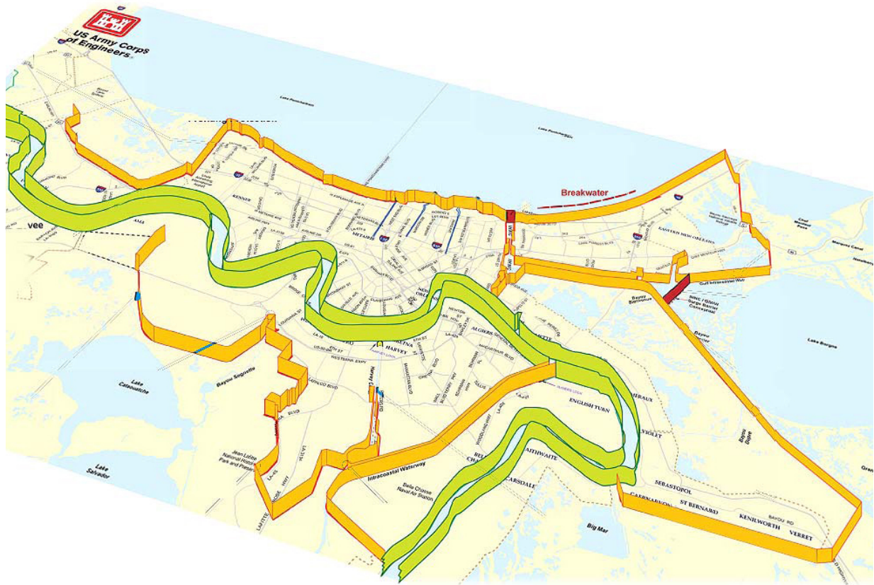
Figure 5-1: A 2008 US Army Corps of Engineers diagram of flood-protection defenses in New Orleans. Green lines represent Mississippi River levees, while orange and red lines indicate storm surge floodwalls, levees, and barriers. The Lake Borgne Surge Barrier is the red line at the eastern edge of the city.
