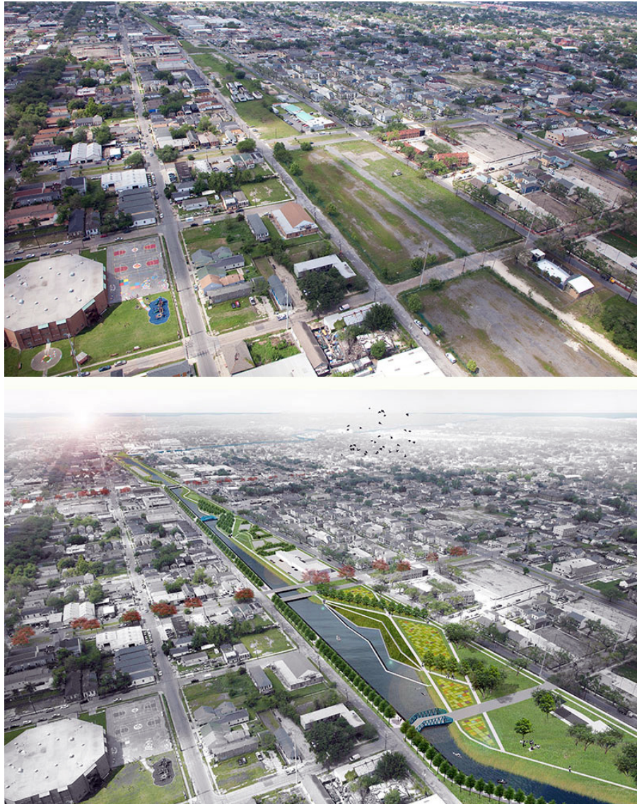
Figure 5-3: The Lafitte corridor (top) reimagined as a greenway (bottom). Images courtesy of Waggonner & Ball Architects.
