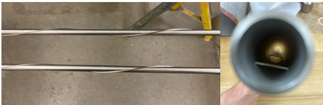
Figure 3-7: Helically wrapped capillary tube on fuel simulator rods (left) and test section capillary tubes for transverse fiber optic temperature sensors (right).
