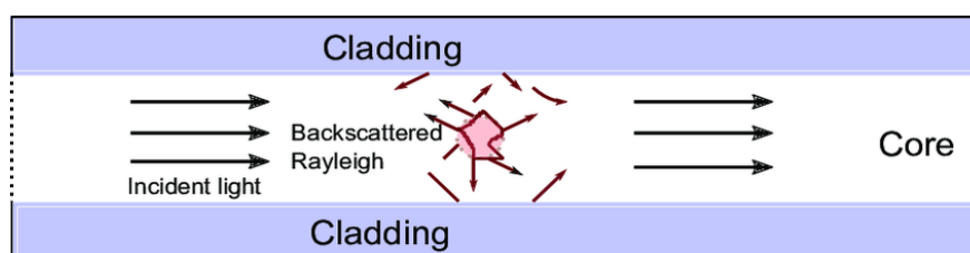
Figure 4-1: Diagram showing optical fiber with Rayleigh backscatter [65], [66].
