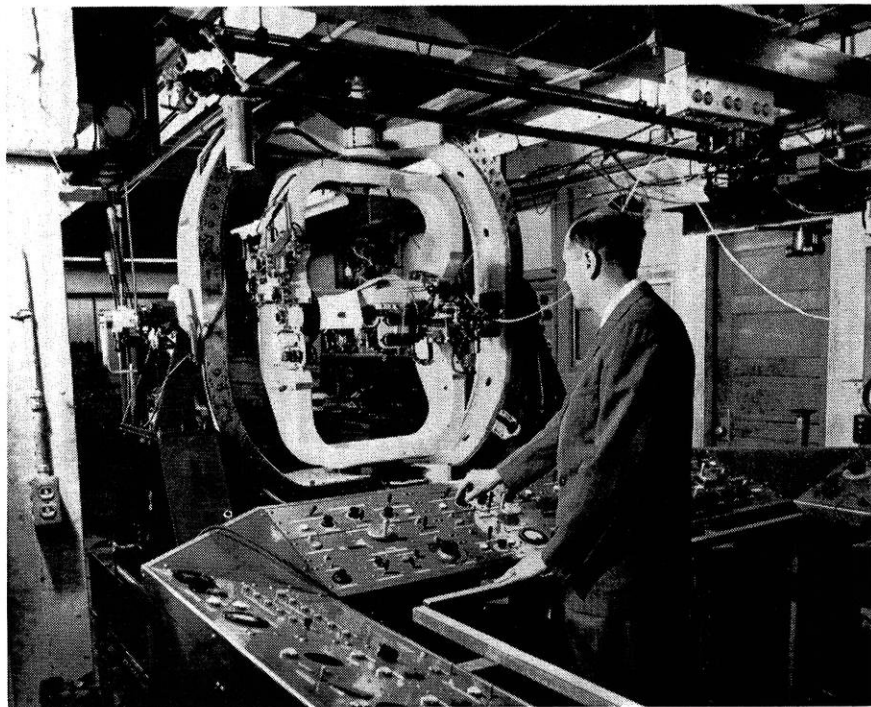
(Photo courtesy Dept. of Defense) Gimbal table and controls for flight test computer.
