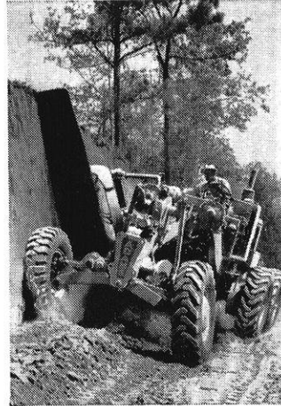
Grader drive axle—Needed: toughness, impact resistance, greatest strength, with least weight. Which alloy?
