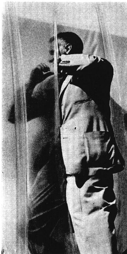
G. T. Schjeldahl, fabricator of the "Schjel-Mile", cut a seven-foot-long gash in the "Scotchpak" skin to prove that small holes won't deflate the building.
