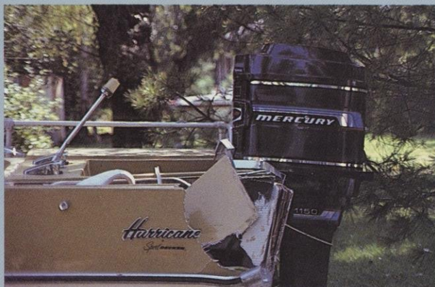
This boat had a white light to mark its stern. But the motor blocked the light from view. And another boat rammed in from behind.
