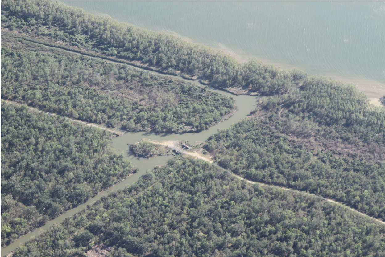
Figure 3. How Mardi Gras Pass has cutoff a road to an oil field. Source .
