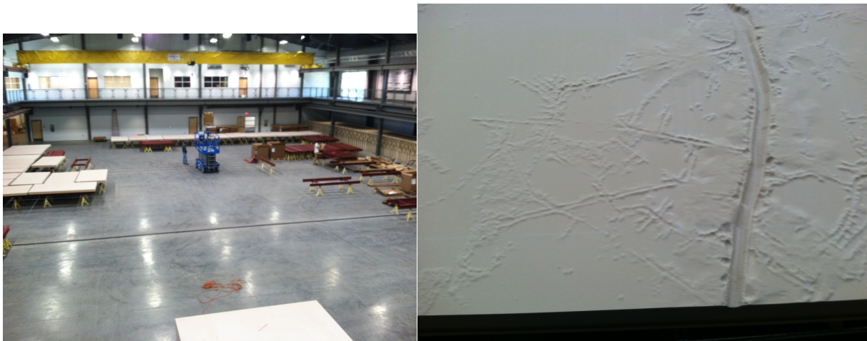
Figure 1. The new Water Campus in Baton Rouge is home to a physical model of the lower Mississippi River. On the left, a view of the model as it is being assembled. On the right, a view of a single panel of the model. The straight lines that are visible are oil and gas canals, and their spoil banks. Source: Author.
