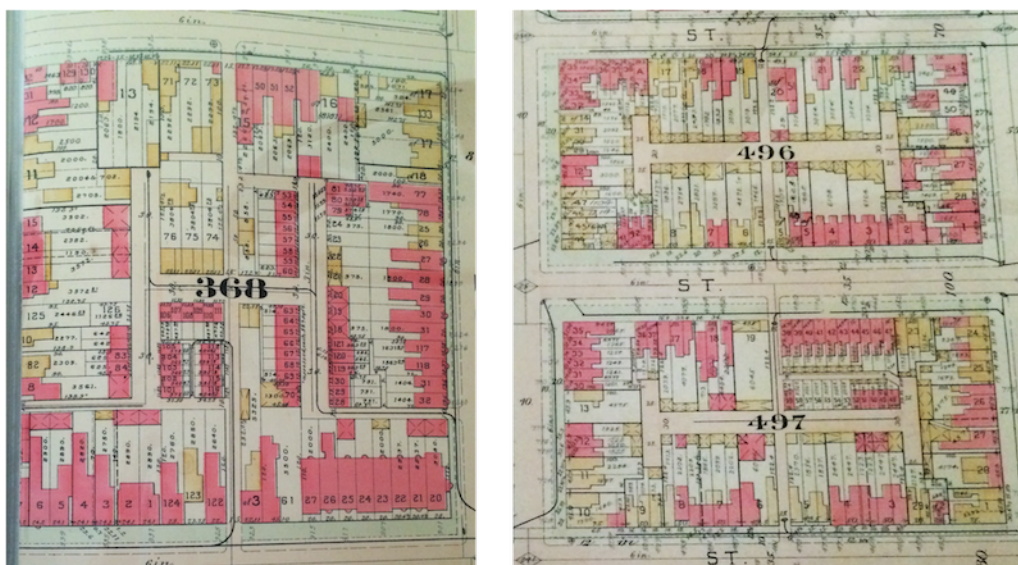
Figure 2. H-shape and I-shape alleys. G.W. Baist, Baist's real estate atlas of surveys of Washington, District of Columbia , 1903.
