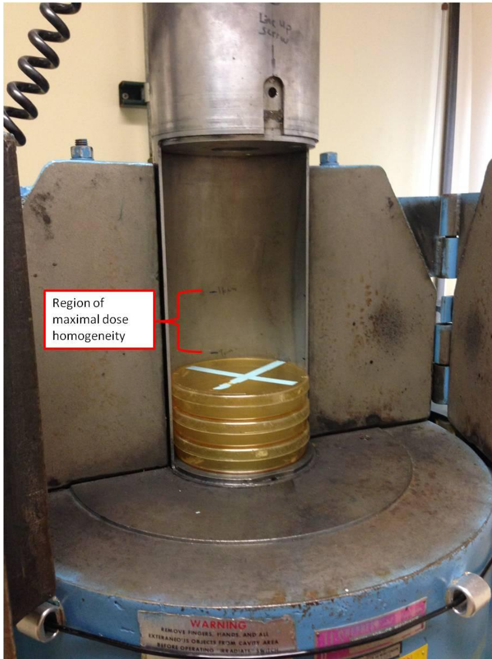
Figure 2.2: Cs-137 pneumatic sample column.
