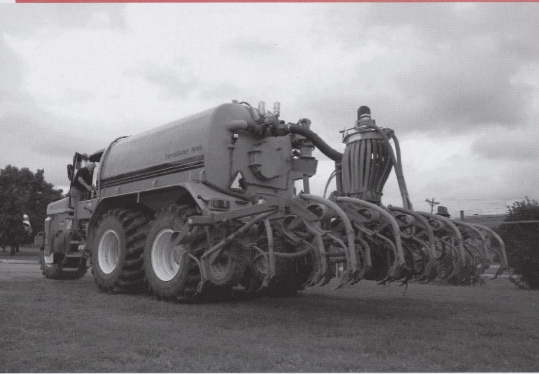
A Terragator with nozzles at back that could inject biosolids into farmland.
