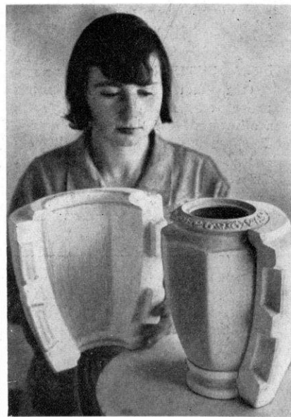
Liquid raw material is poured into mold; allowed to stand for about two hours until shape of vase is formed.
