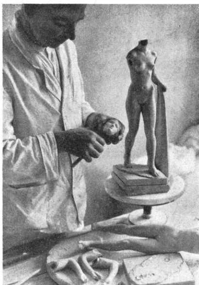
After figurine parts are removed from molds separate pieces must be carefully joined in preparation for firing.
