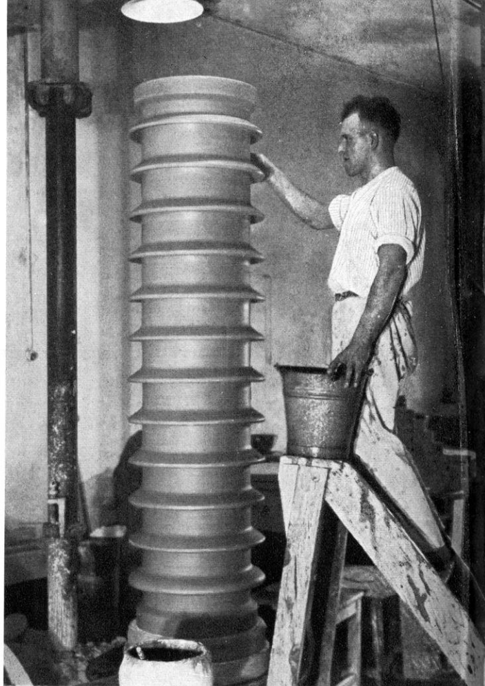
Making insulators here shown, as well as a wide variety of other technical products is an important part of ceramics
