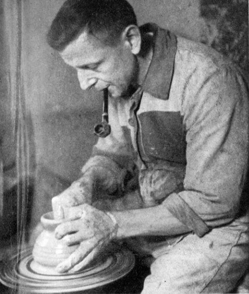
Three steps used since medieval times in shaping a vase on a potter's wheel (Walther Plant, Bad Koenig, Odenwald).
