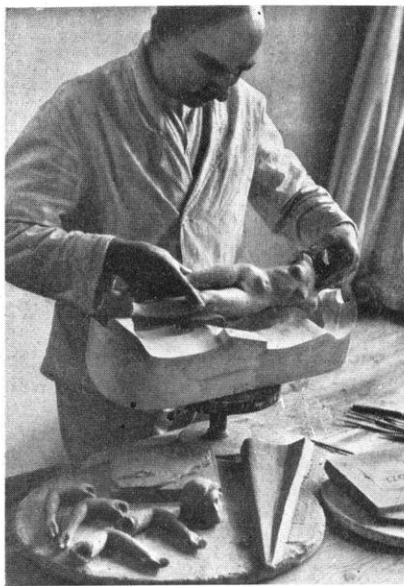
After figurine parts are removed from molds separate pieces must be carefully joined in preparation for firing.
