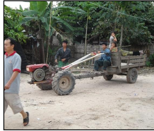
Figure 5.2: Paddy tilling machine modified to serve as a transportation vehicle. Photograph by P. Vue.
