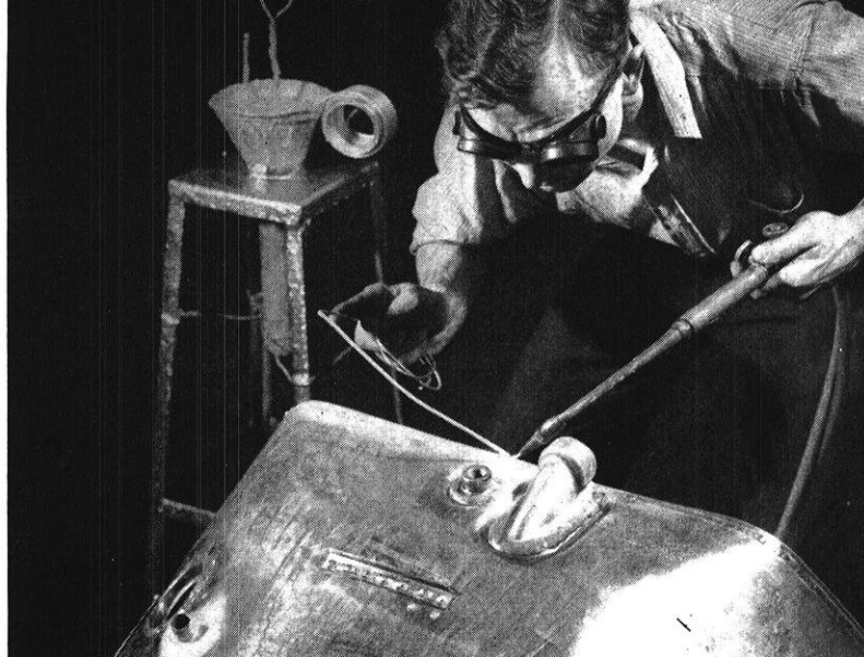
Cast fittings are welded to an oil tank by means of an oxy-acetylene flame and a protective flux. The baffle sheets within the tank are joined to the shell by spot welds.
