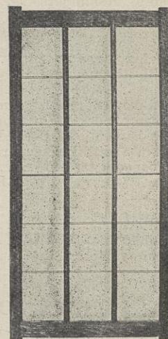
Size 3 ft. by 6 ft. for 3 rows 10 in. lapped glass.
