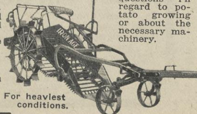
Four Row 55 Gallon Tank 22 in Elevator 32 in. Wheels
