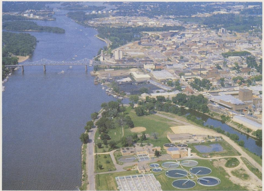
This sewage plant at La Crosse was upgraded to secondary treatment status in 1972. It handles about 12-million gallons per day but has a capacity of 20-million. Eighty-five per cent of all contaminants must be removed before effluent can be discharged. The Black and La Crosse Rivers come into the Mississippi at the top of the photo. Most water in the basin is getting progressively cleaner as more plants like this come on line. However, the attack on nonpoint pollution has only just begun. Photo by Dave Weitz
