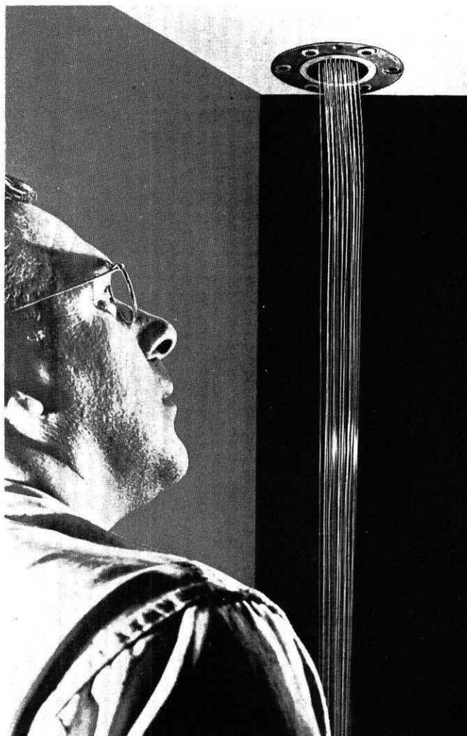
The birth of "Dacron" filaments. From tiny holes in this spinneret are extruded fine filaments of "Dacron". All of the filaments shown here will be wound together to form a single strand of yarn.
