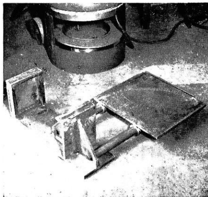
Motor Swing Base is fabricated at low cost from tubing and steel plate. Welds are made with "hidden-arc" process in agglomerated flux, using Manual Lincoln weld.
