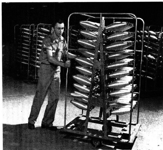
From the final packaging machine, carts of "Orlon" in the form of continuous filament yarn go to the inspection table for a thorough examination.
