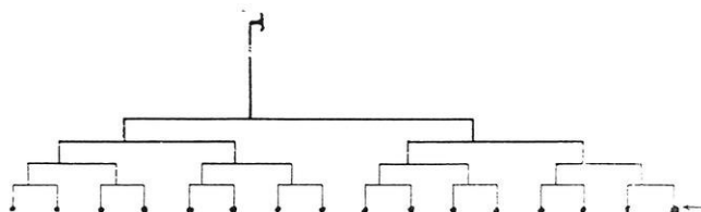
FIG. 18. THE M-F TUBE. This illustrates forward compensation. Each junction point divides the length of the horizontal tube in the ratio of 65:35, the ratio of the velocity of sound in air to that in water.
