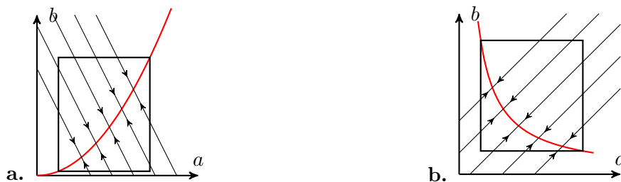
Figure 3.1: Construction of a rectangular invariant region for the reversible reaction m_1A + n_1B \rightleftharpoons m_2A + n_2B for the cases a. \bar{m} = m_1 - m_2 , \bar{n} = n_2 - n_1 nonzero and of the same sign; b. \bar{m}, \bar{n} nonzero and of different signs.
