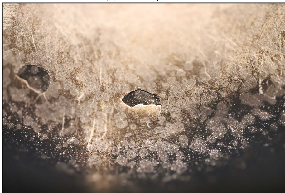
(b) View close to a delamination spot
