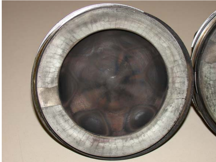
Figure 2.2: Top view of a Caterpillar heavy-duty piston showing spallations and cracks of a glass sealed coating at the squish area. Taken from Beardsley [68, 70].
