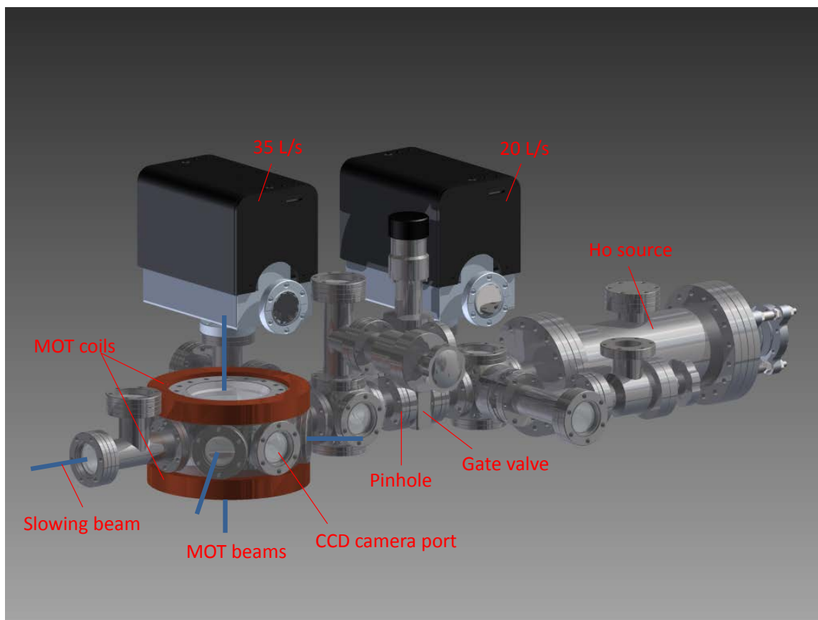
Figure 2.2 The vacuum system used for a majority of the experiments. The system is separated into two sections, the source region and the science region. The holmium source is located at one end. It attaches directly to a chamber with viewports available for spectroscopy and for vacuum connections. There is a gate valve separating the two regions. On the other side of the gate valve is another section available for transverse cooling, spectroscopy, and vacuum connections. The trapping region is inside the spherical octagon. A tee is opposite the source to hold a mirror to support the slowing beam.
