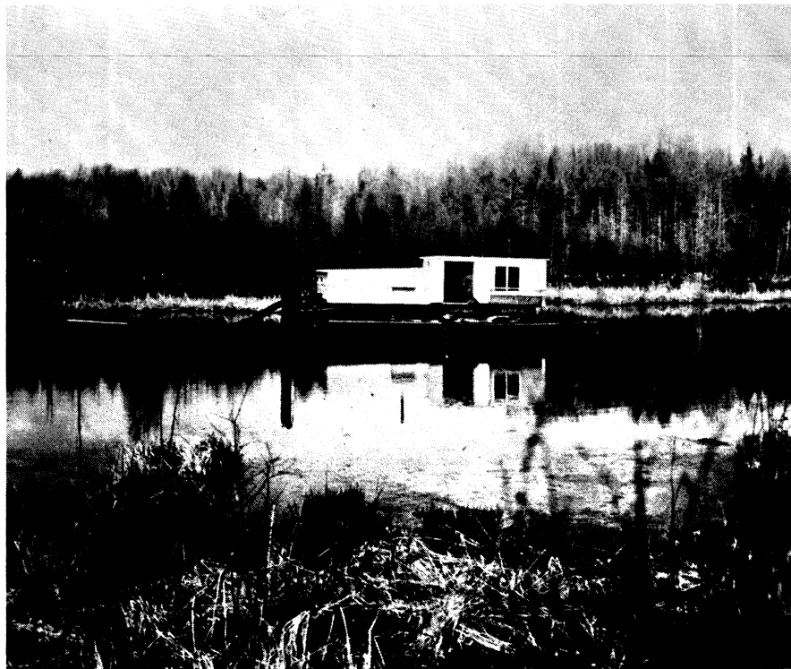
The DNR owns two dredges such as this one. It is equipped with a 6-inch intake pipe and powered by a 140 hp engine.
