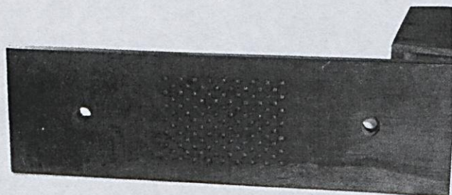
Figure 4 (above bottom). The hatchel board underside. Note the measured arrangement of the spikes.
