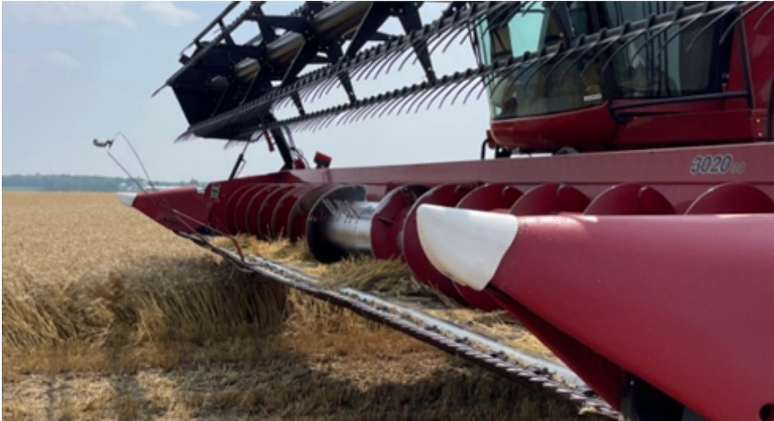
Figure 3.3: Action camera mounted on the harvester capturing video during the harvesting process. The video data is used to validate the trained models' performance in detecting pre-harvest loss in real-time field conditions.
