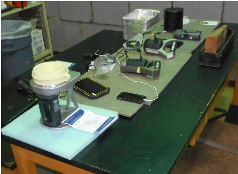
Figure 1.2: Handheld NIR sensors evaluated in this study. From left to right: NeoSpectra (1350–2550 nm, Si-ware Systems Inc., Cairo, Egypt) placed on a turntable; Trinamix (1450–2450 nm, TrinamiX Inc., Ludwigshafen, Germany); and a SCiO Cup (740–1070 nm, Consumer Physics Inc., Tel Aviv, Israel). Photo credit to Dr. Jerry Cherney.
