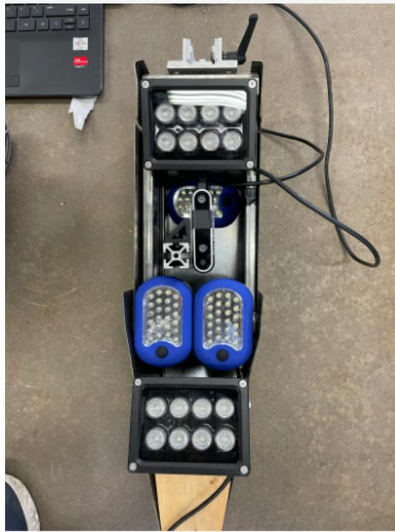
Figure 3.2: Fabricated UGV snout equipped with a RealSense D435i camera, a 15 cm LED Light Bar, and an IR Illuminator (850 nm). The snout provides protection for the camera and artificial lighting for improved image quality under various lighting conditions.
