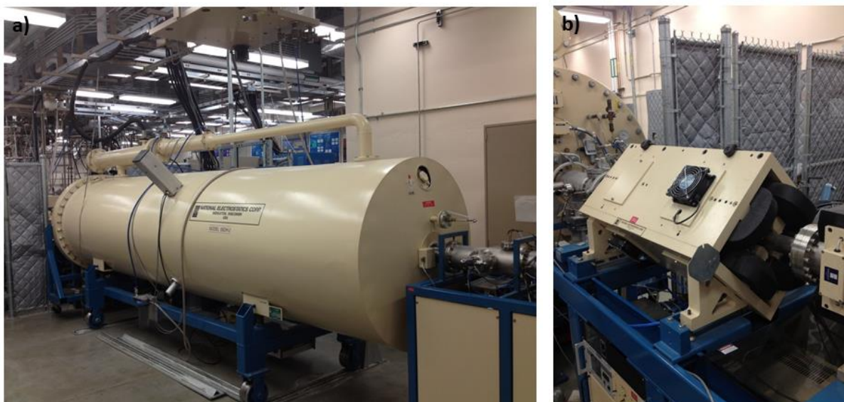
Figure 3-6: EMSL accelerator (a) accelerator tank (3MV Tandem Van Der Graaff accelerator) and (b) set of quadrupole magnets in the high energy part of the beam.
