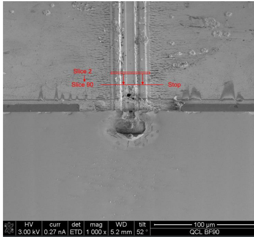
Fig 3.6 SEM image of the BH device that was previously mounted epi-down on copper with indium, experienced failure, and shows catastrophic mirror damage directly over the active region.
