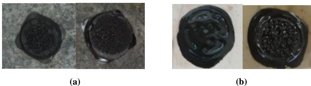
Figure 4-39. Typical Failure Modes in the BBS (a) Cohesive Failure (b) Cohesive and Adhesive Failure.
