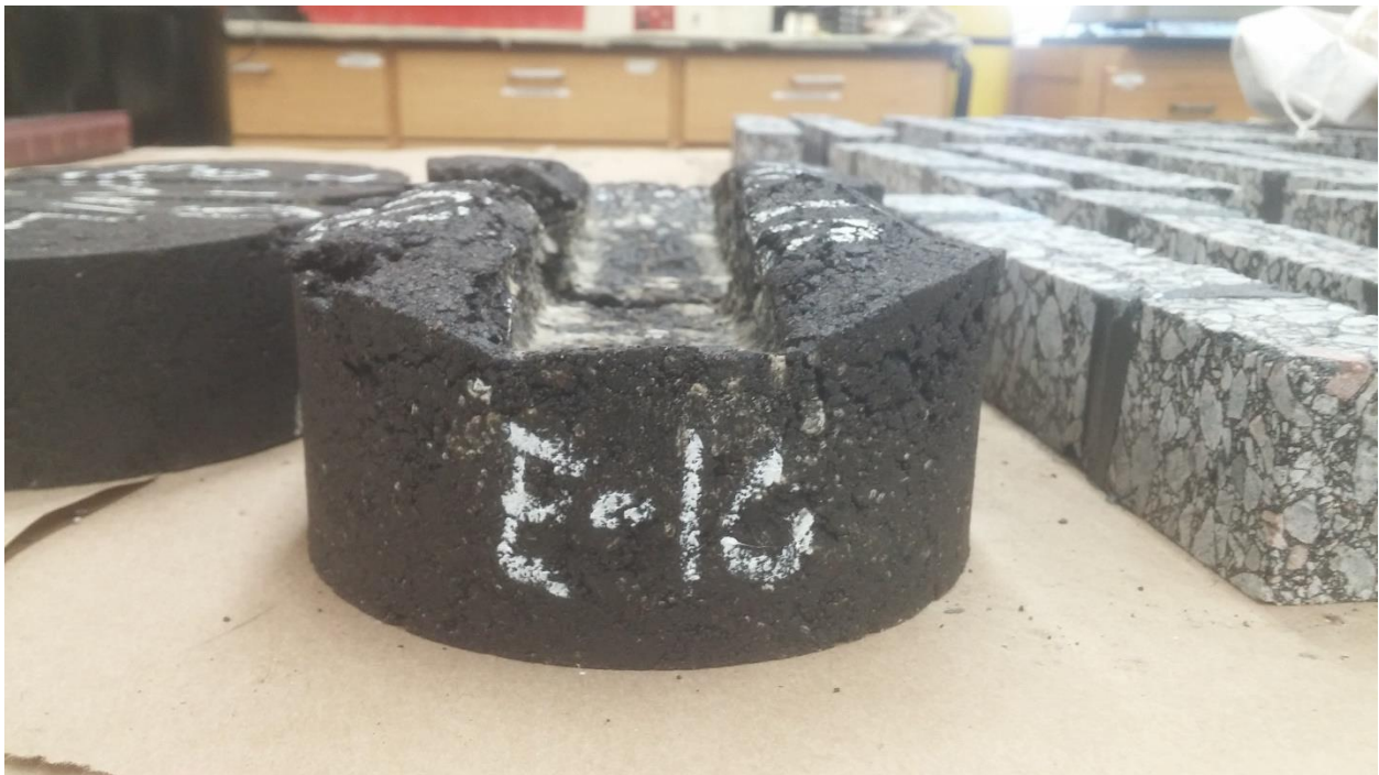
Figure B-2. The E-10 Mix in Experiment 1 and 2 after Dry HWT Testing.
