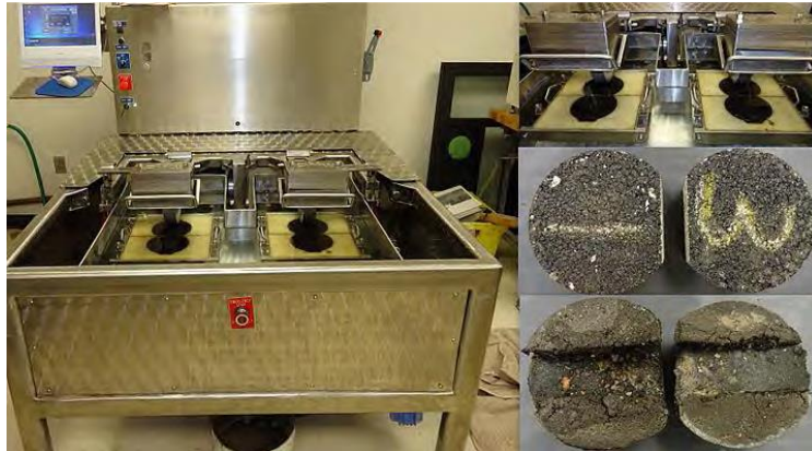
Figure 2-3. (Clockwise) Final Test Setup of Hamburg Wheel Tracking Device, Specimens under the Wheel Load, Specimens Ready for Testing in HWT Device, and Failed Specimens with High Rut Depth (Rahman and Hossain 2014).
