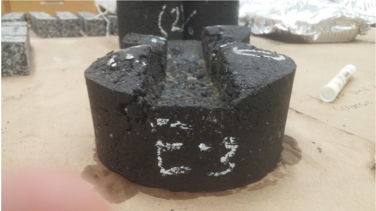
Figure B-1. The E-3 Mix in Experiment 1 and 2 after Dry HWT Testing.
