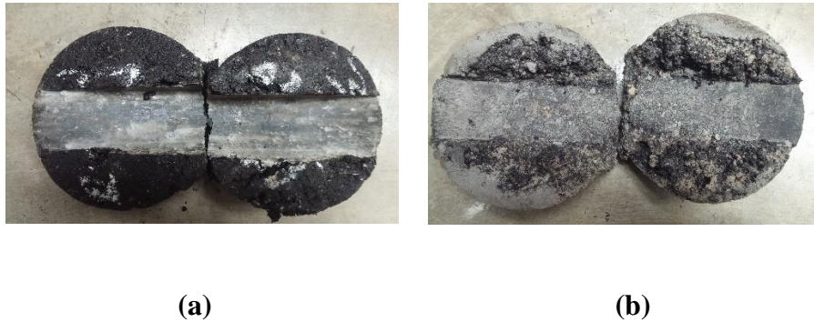
Figure 4-34. Failure of HWT Samples on Running in (a) Dry Condition (b) Wet Condition
