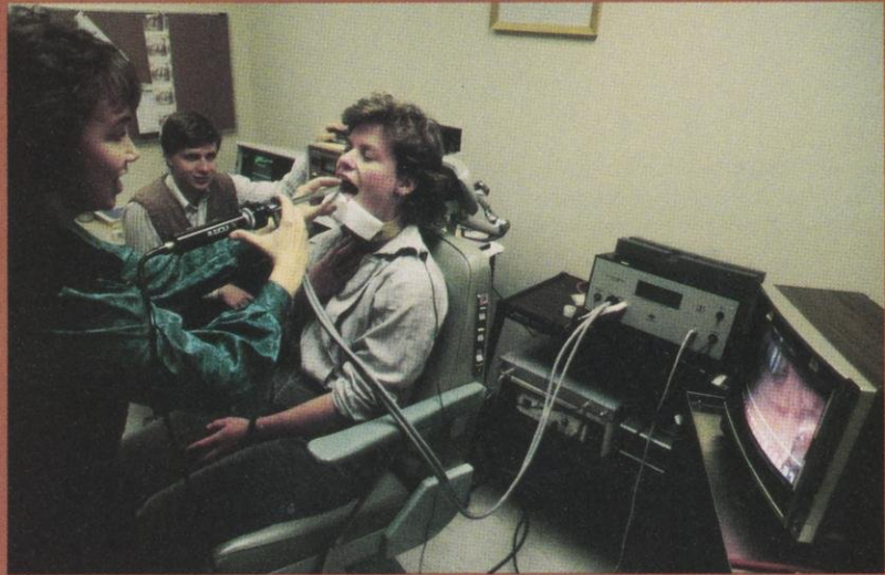
The videostroboscope is a pencil-sized camera which records laryngeal action at thirty frames per second. The system was largely developed by Bless and Paul Milenkovic (in background).
