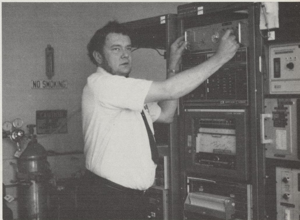
Above, a monitor in Milwaukee, part of the air program network. It monitors fine particles which can penetrate lungs. Below, air monitoring supervisor Ed Miller, with lab equipment used to assure the accuracy of air monitors in the field.
