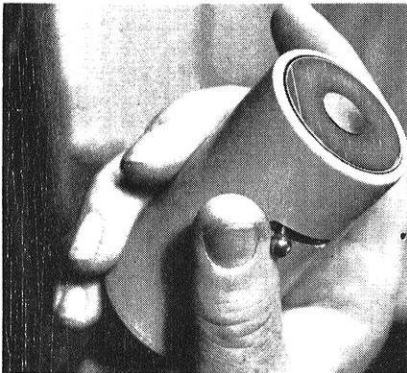
New electronic artificial larynx utilizes a modified telephone receiver which transmits sound through flesh into person's throat.
