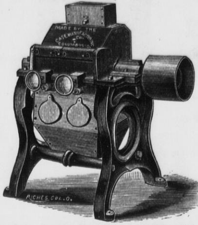
Single Break Machine, capacity 5 to 60 bushels per hour.
