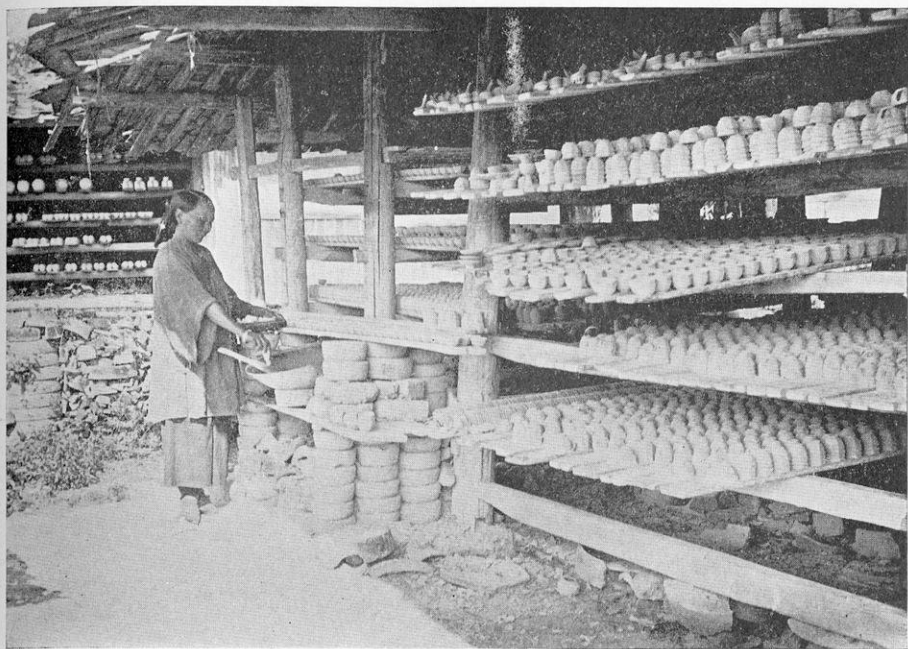
Drying the freshly moulded ware
