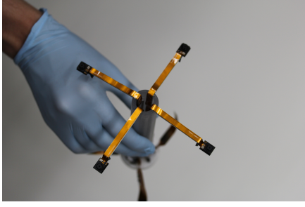
(a) Trocar-based Camera Array
