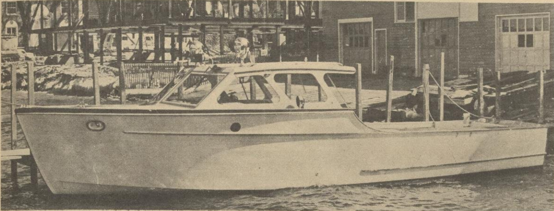
NEW CRUISER —This latest addition to the rescue station is powered by twin V-8 Chrysler engines of 500 horsepower. It can reach speeds of over 40 miles per hour. It is also equipped with a police radio to give lifesaving crews direct communication with campus police and other local enforcement agencies.
